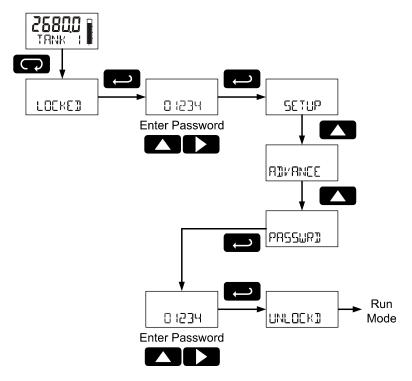
If the correct five-digit password is entered, the meter displays the message LINLOCKI (unlocked) and the protection is disabled until a new password is programmed. If the password entered is incorrect, the meter displays the message LOCKEI and returns to Run Mode. To try again, repeat the above procedure.
