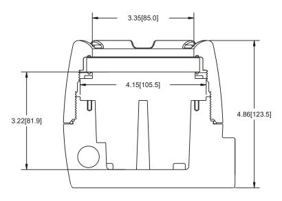
Figure 10. Enclosure Dimensions - Side Cross Section View
