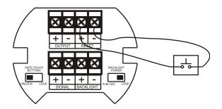
Figure 5. External Alarm Reset/Acknowledge Connections
