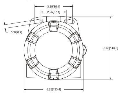
Figure 9. Enclosure Dimensions - Front View
