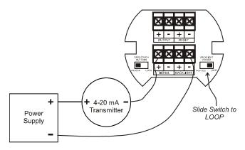
Figure 3. Connections with Loop-Powered Backlight
