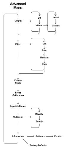
\*Access by holding Right/Reset for 3 seconds
