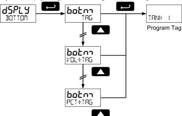
The fully alphanumeric values for the tag are set using the **RIGHT** button to select the digit, the **UP** and **RIGHT** arrow buttons to select the digit reading, and the **ENTER** button to confirm and select the next digit.
