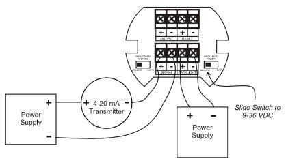
Figure 4. Connections with Externally-Powered Backlight
