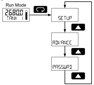
Hold **MENU**, at any time, to exit and return to *Run Mode*. Changes made to settings prior to pressing **ENTER** are not saved.
