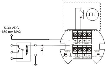
Figure 7. Output Connections
