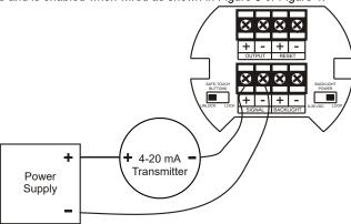
Figure 2. Connections without Backlight
