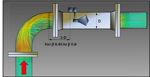
Figure 7. Cone meter straight run location
