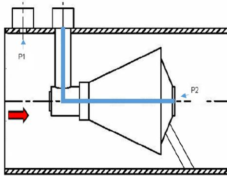
Figure 5. Horizontally Mounted Cone Type Meter (Normal)
