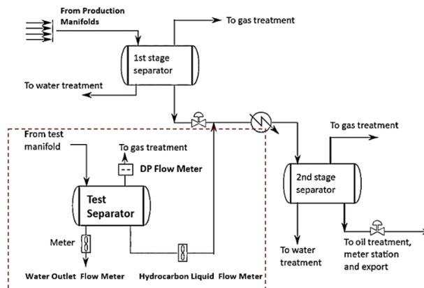
Figure 1. Typical Liquid & Gas Hydrocarbon Separation System.
