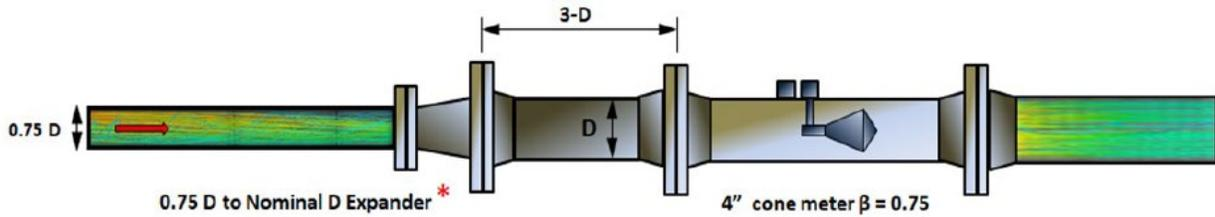
Figure 9. Concentric Expander Installation (ISO 5167-5)
