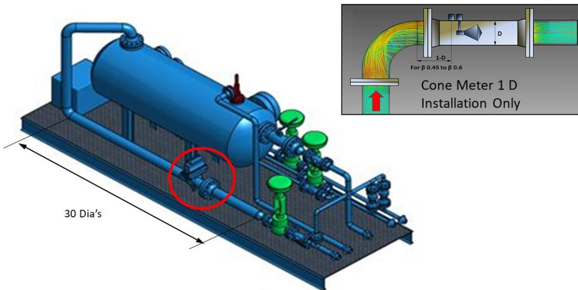
Figure 10. Test Separator Comparison Regarding Installation Length.
