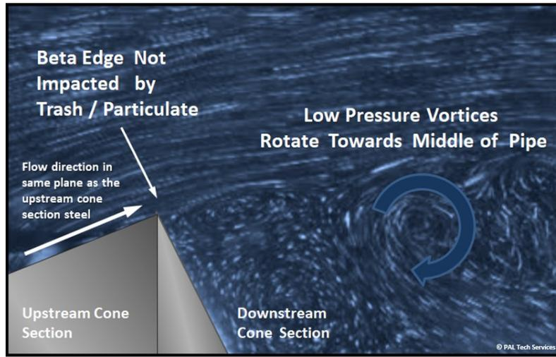
Figure 11. Cone meter Beta Edge Location and Contour
