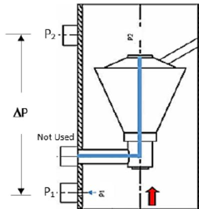
Figure 6. Vertically Mounted Cone Meter (Special)
